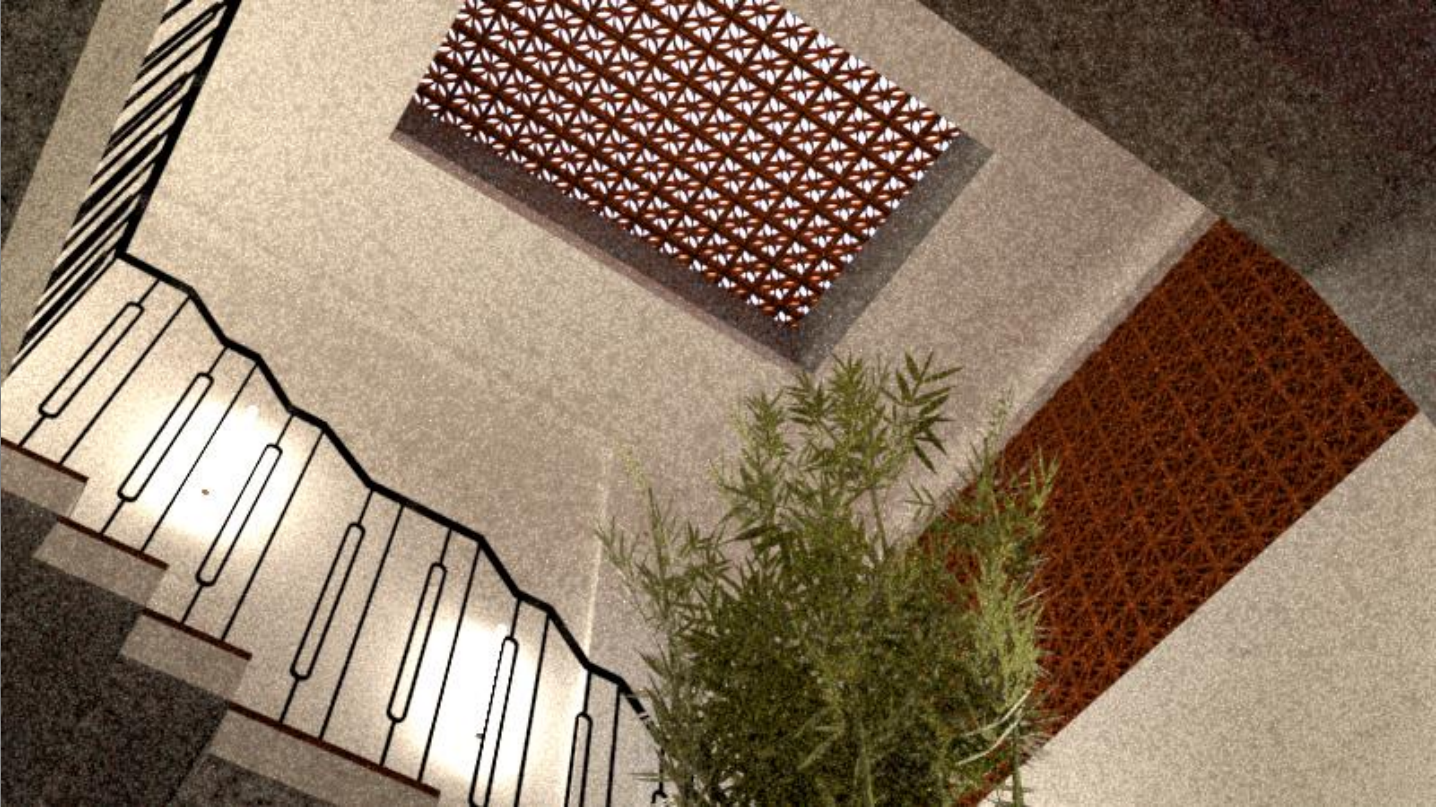
Skylights above staircase for continuous light intake & cutoff of heat gain as no much human interaction
